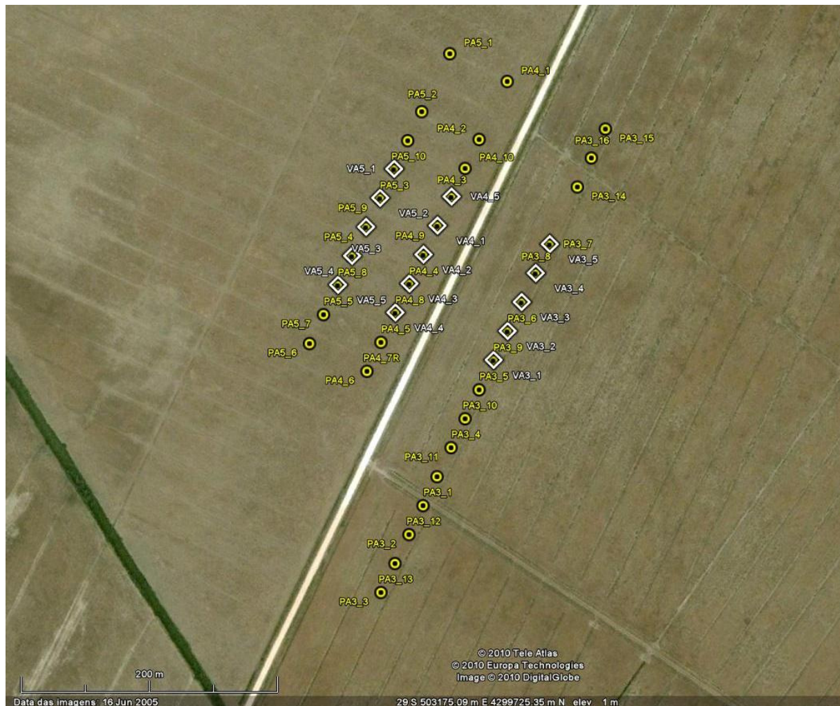
Figure 4.3 – VES (yellow circles) and TEM (white squares) soundings disposition at the field. North is up at this image (adapted from Google images).
