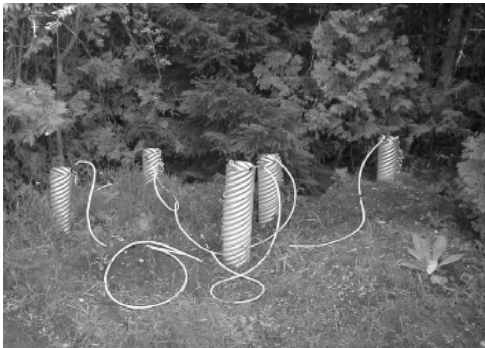
Electrode farm at the test site. Multiple electrodes reduce the contact resistance.
