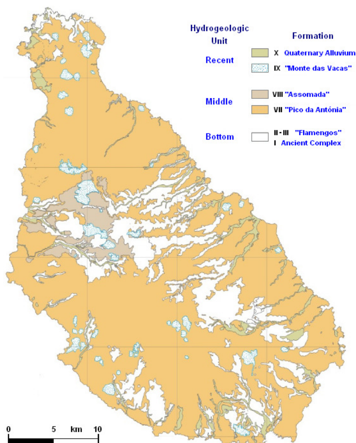
Figure 6.19 – Hydrogeologic Units at Santiago. (Modified from Serralheiro, 1976a).
