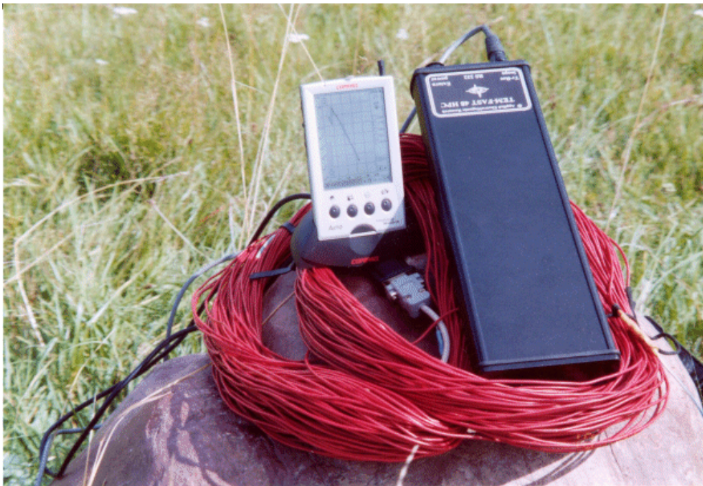
Figure 2.13 – TEM FAST 48 set with main unit (103 mm × 27 mm × 310 mm), loop cables and small pocket personal computer, (original photography from AEMR).
